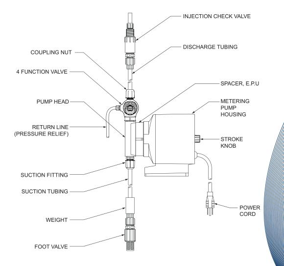
Metering Pump Component Diagram
